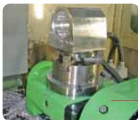
Usinage 5 axes CNC
